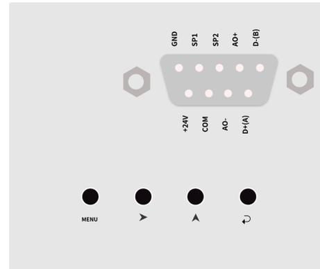
The top of CFV106 consists of a DB9 female socket and 4 touch buttons. Power supply, data communication, analog output, and control point switches are all integrated into the DB9 data interface, as defined in Part 5.
